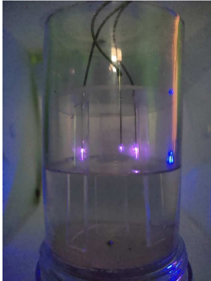
Fig. 4. Typical plasma generated during water treatment process
