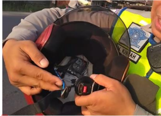
Figure 8. Electronic devices embedded at helmet unit.
