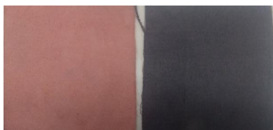
Figure 7. The color cellulose fiber result on a cotton cloth after the fixation process
