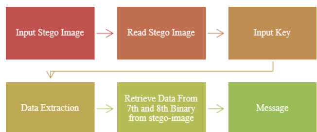
Fig 6. Message Extraction Process
