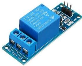
**Gambar 3.** Relay Module 5 Volt 10A Water inlet valve
