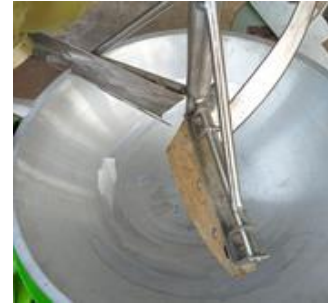
Figure 3b. Agitator blade after modification
