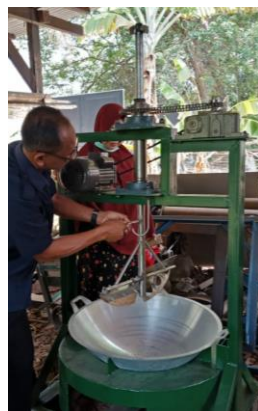
Figure 2. Brown sugar semi-automatic cooking machine
