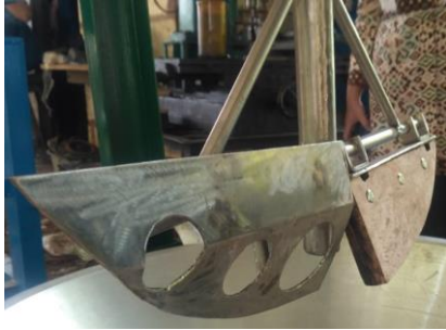
Figure 3a. Agitator blade before modification
