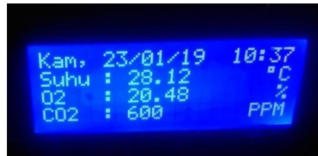
Figure 4. Display Data to 20x4 Character LCD
