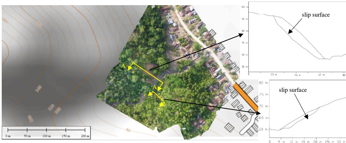
FIGURE 6. The cross section of Sedayu landslide
