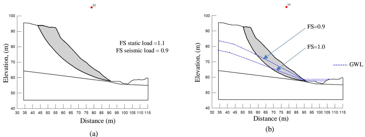
**FIGURE 8.** earthquake or groundwater induced slope failure
