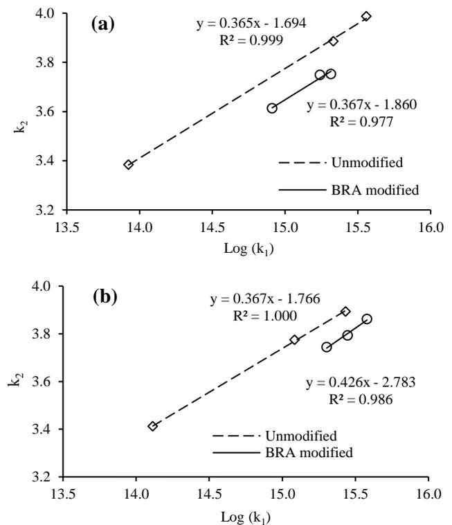
Fig. 10 The relationship between  $k_1$ - $k_2$  for unmodified and BRA-modified asphalt mixtures using (a) classical approach and (b) energy-stiffness ratio approach.
