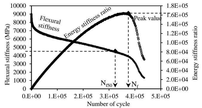
Fig. 5. Energy stiffness ratio versus loading cycles (for specimen tested at  $20^\circ\text{C}$  and  $400\mu\epsilon$ ).
