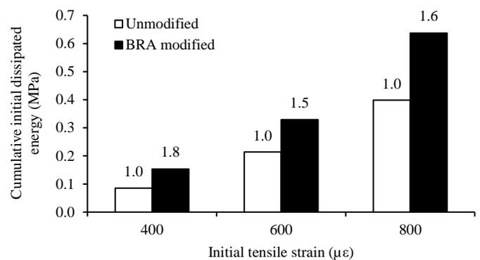
Fig. 14. Cumulative initial dissipated energy for asphalt mixtures.
