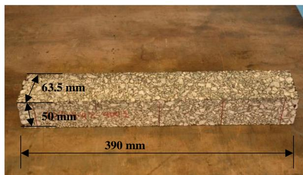
Fig. 3. Final beam specimen.
