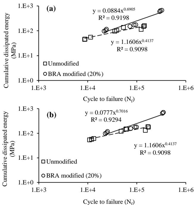
Fig. 13. Relationship between cycle to failure and cumulative dissipated energy using (a) classical approach and (b) ER approach.
