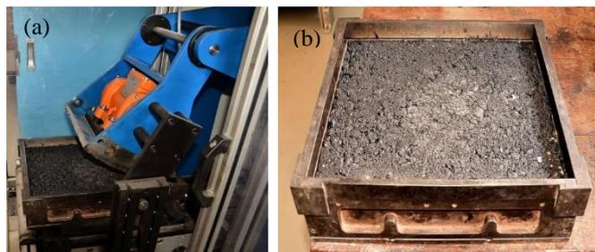
Fig. 2. Compaction process for the slabs in the flexural bending test.
