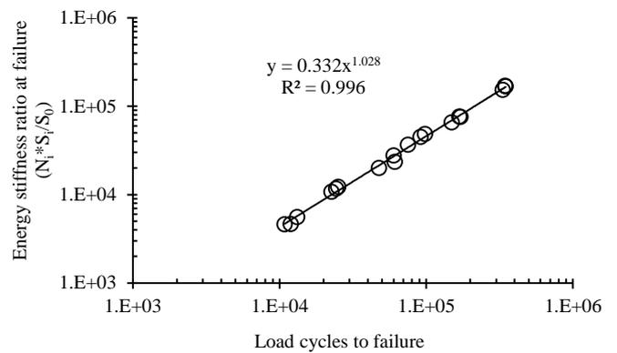
Fig. 7. Energy stiffness ratio at failure vs load cycles at failure for controlled strain.
