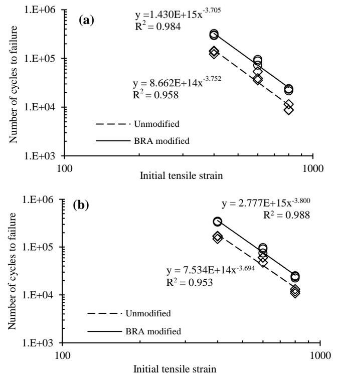
Fig. 8. Fatigue characteristics of unmodified and BRA modified asphalt mixtures using (a) classical approach and (b) ER approach.
