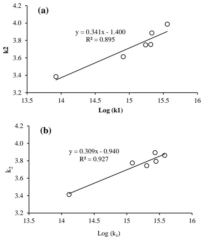
Fig. 9. The relationship between  $k_1$ - $k_2$  for all asphalt mixtures using (a) classical approach and (b) ER approach.
