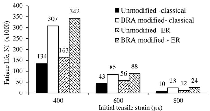
Fig. 6. Mean fatigue life of asphalt mixtures.
