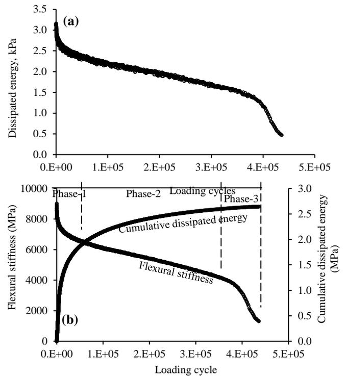
Fig. 12 Typical results of fatigue test (a) evolution of dissipated energy per cycle, (b) progression curve of flexural stiffness and cumulative dissipated energy.
