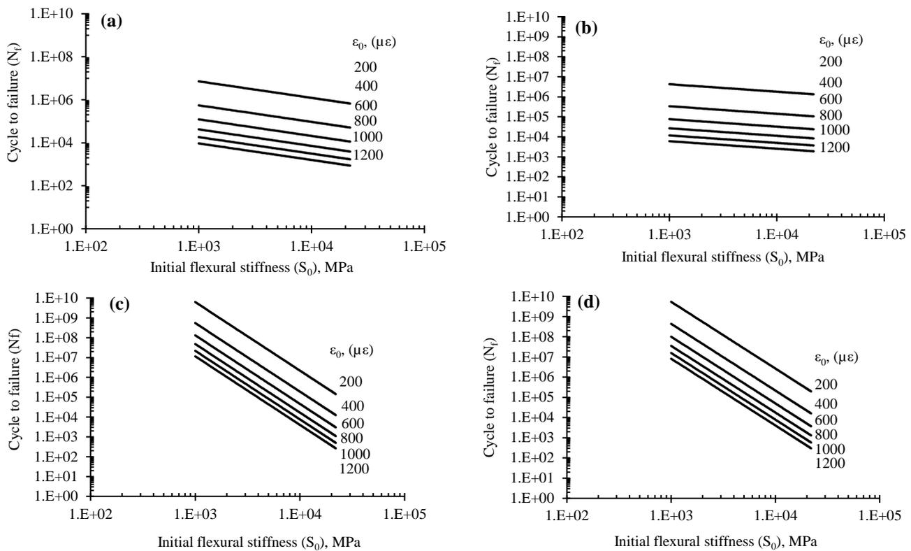
Fig. 11. Strain-stiffness relationship between  $N_f$ ,  $\epsilon_0$ , and  $S_0$ : (a) Unmodified (classical), (b) Unmodified (ER), (c) BRA-modified (classical), and (d) BRA-modified (ER).
