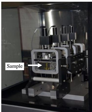
Fig. 4. Set-up of the repeated flexural bending test.
