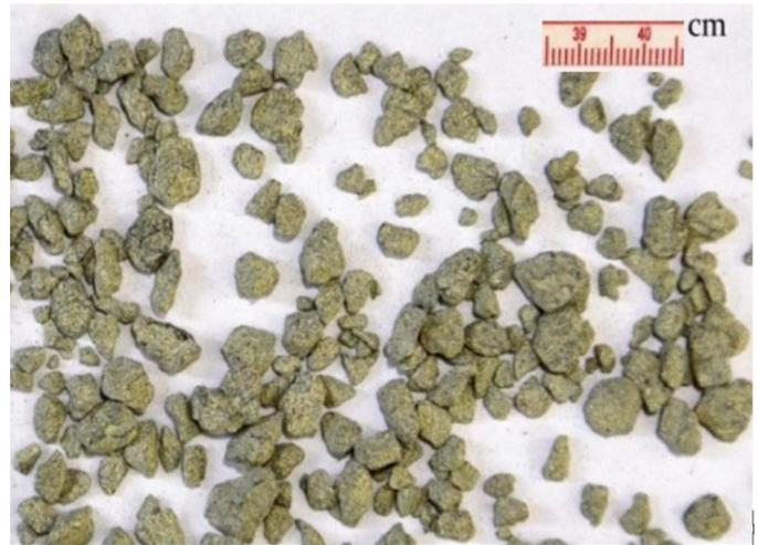
Fig. 1. The form of granular BRA modifier binder (pellets).
