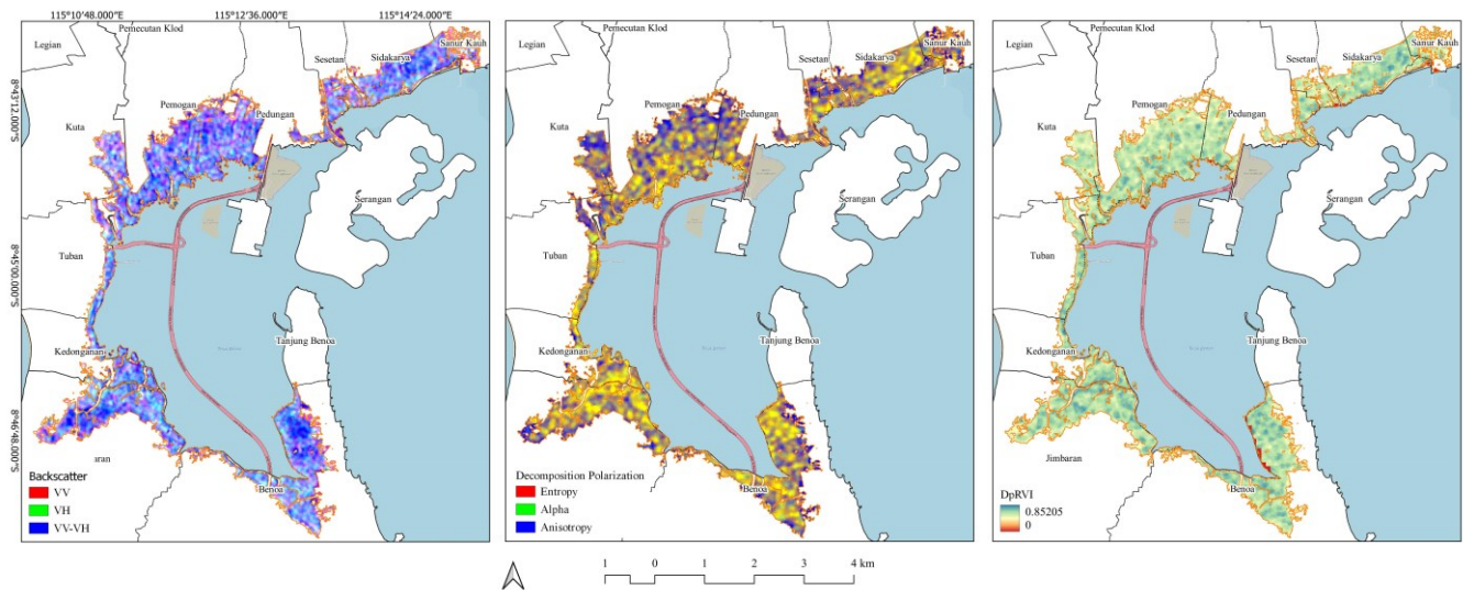
Figure 2 Processed Sentinel -1 data to backscatter, decomposition polarization and DpRVI
