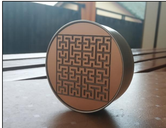
Figure 2. Microstrip Hilbert fractal 4 th order antenna.
