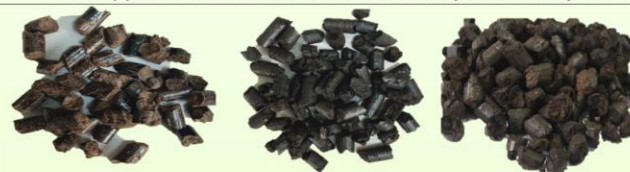
a. Non-torrefied Pellets b. Torrefaction pellets use electric furnaces c. Torrefaction pellets use COMB reactor
