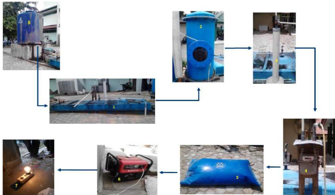
Figure 1. Tools and equipment used in the study, from biogas production to generator testing: 1. Wet anaerobic digester (5 m 3 ); 2. Bio-filter scrubber; 3. Pressure expansion (dryer); 4. Biogas flowmeter; 5. Biogas storage; 6. Generator engine 750-W; 7. Load; 8. Substrate storage tank (5 m 3 ).
