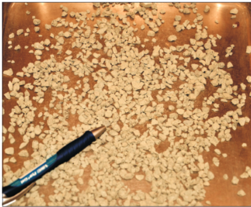
Fig. 2. Pellets of granular BRA modifier binder
