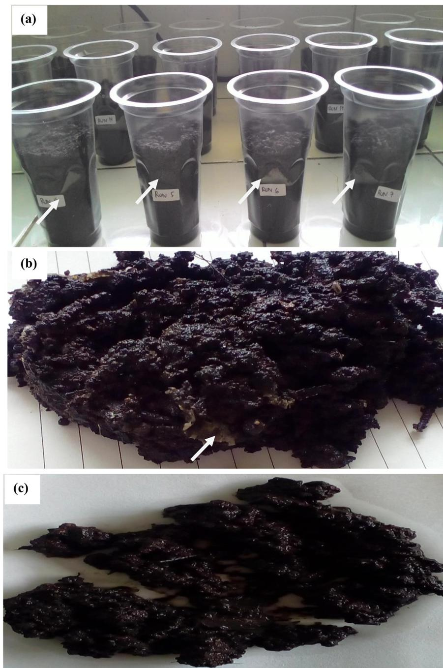
**Figure 3.** (a). Biodegradable film planted in pots filled with soil, the film sheet is clearly visible; (b). Observation of the biodegradable film test results in the first week still send the film sheets that have not been degraded; (c). Observation of the biodegradable film test results in second week, no film sheets were visible.
