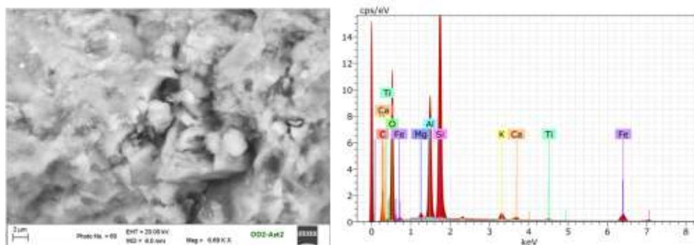
Figure 6. SEM analysis on clay shale (OD2-Ast2)
