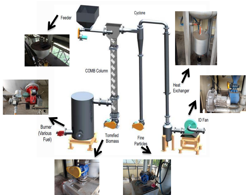
Gambar 6. Bagian-bagian reaktor Counter Flow Multi Baffle (COMB).
