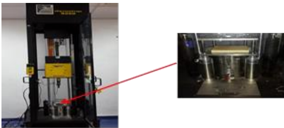
Fig.1 Low-velocity impact test conducted in this study.
