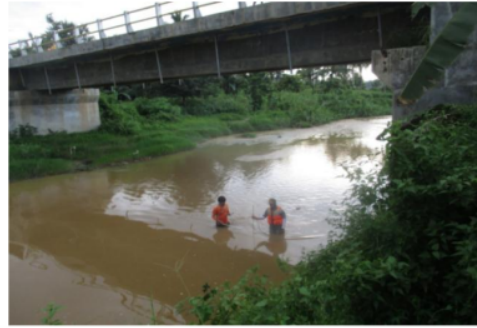
Figure 5. Discharge measurement at Giri Tunggal Bridge, Way Wayah River
