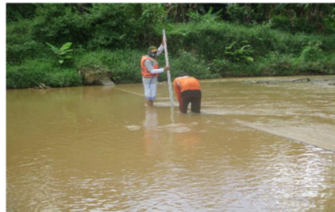
Figure 4. Discharge measurement at Madaraya Bridge, Way Wayah River
