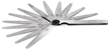
**Gambar 8.** *Feeler gauge*- alat pengukur *clearance* dudukan *valve*
