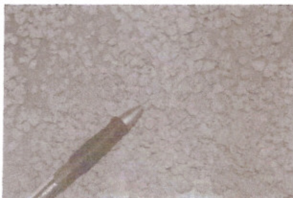
Figure 1. The form of granular BRA modifier binder.
