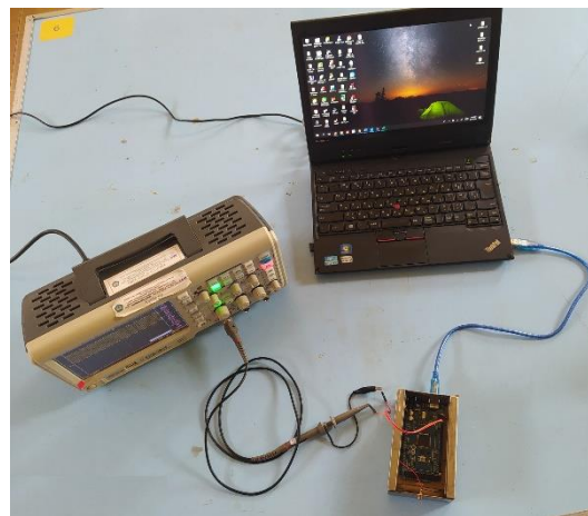
Figure 2. Circuit to test the software’s output.
