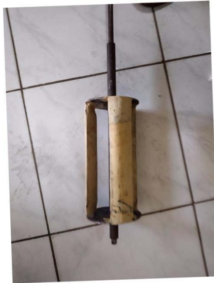
Figure 8. Model of hydrokinetic turbine with tree blades
