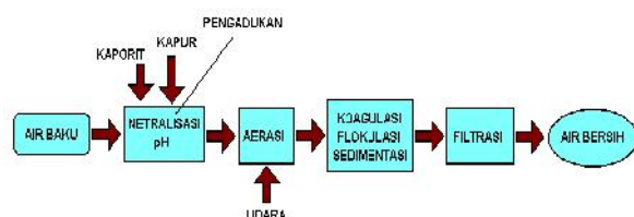
Gambar 1. Diagram Proses Pengolahan Air Gambut (Google Images, 2015)
