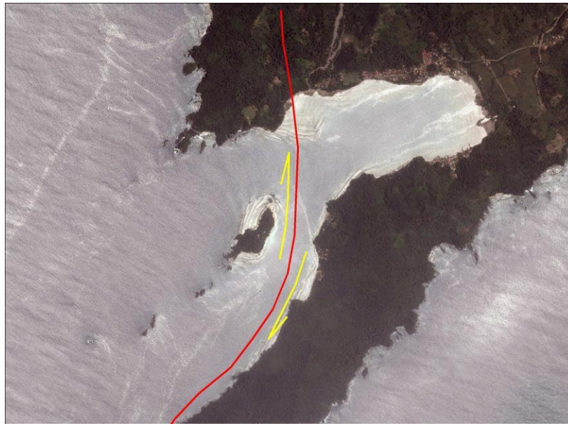
Figure 6. Reconstruction of fault shear obelique in the Kiluan bay.
