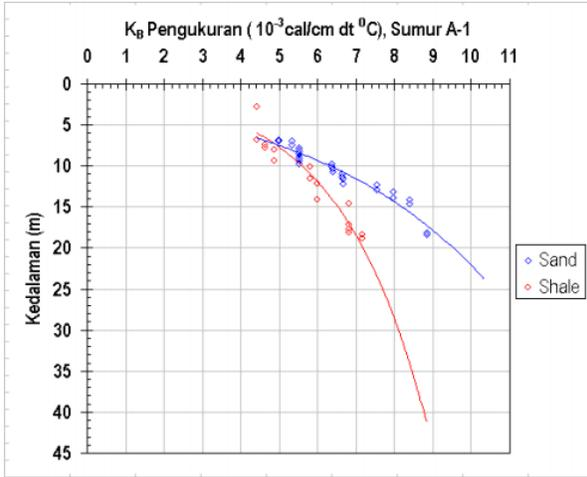
FIGURE 1. Relationship between thermal conductivity of rocks measurement and depth for well A-1
