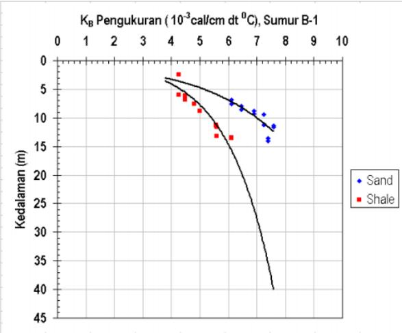
FIGURE 3. Relationship between thermal conductivity of rocks measurement and depth for well B-1
