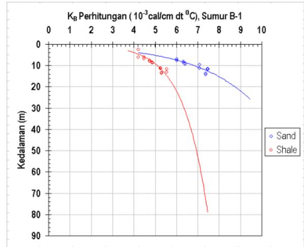
FIGURE 4. Relationship between thermal conductivity of rocks calculation and depth for well B-1
