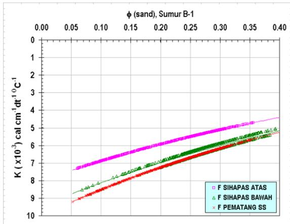
**FIGURE 7.** Relationship between thermal conductivity of rocks measurement and sand porosity for well B-1
