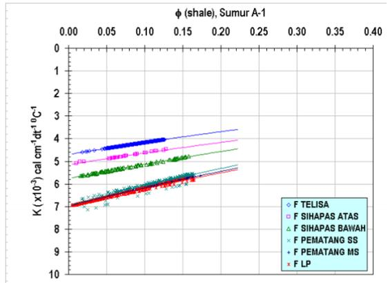
FIGURE 6. Relationship between thermal conductivity of rocks calculation and shale porosity for well A-1
