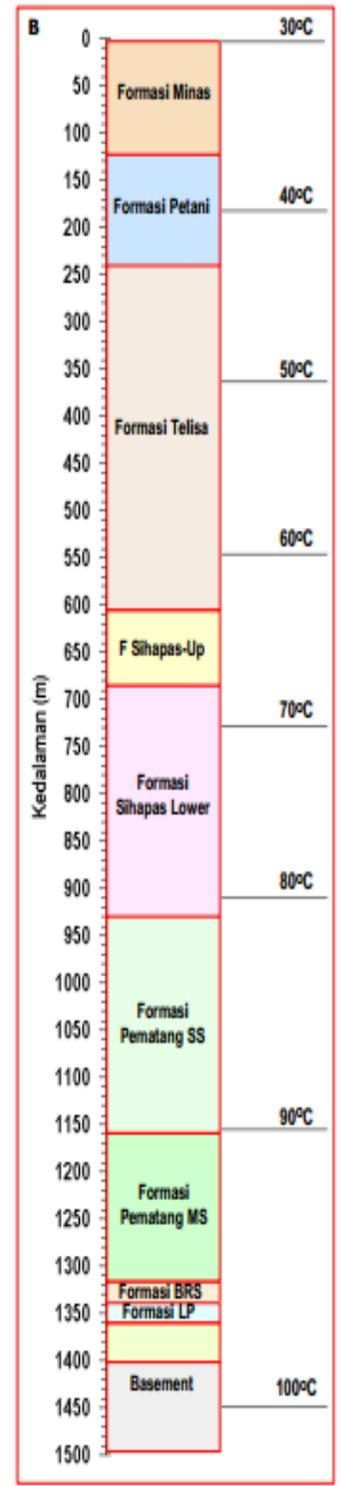
FIGURE 9. Formation temperature for A-1 from thermal conductivity of rocks measurement (A) and calculation (B)
