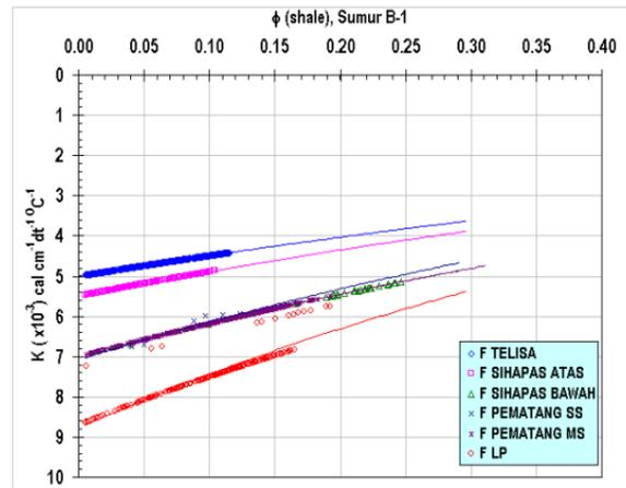
**FIGURE 8.** Relationship between thermal conductivity of rocks calculation and shale porosity for well B-1
