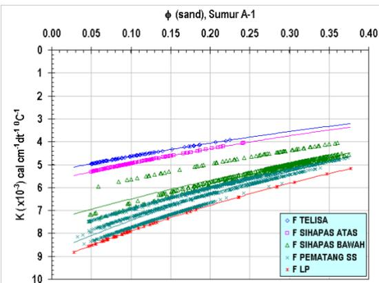
FIGURE 5. Relationship between thermal conductivity of rocks measurement and sand porosity for well A-1
