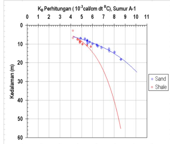
FIGURE 2. Relationship between thermal conductivity of rocks calculation and depth for well A-1
