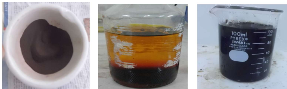
Figure 1. (a) iron ore sample sieve 230 mesh, (b) iron ore with HCl solution, and (c) ZnFe 2 O 4 solution.
