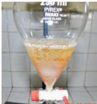
5 Fig. 1: Formation of soap during transesterification of rubber seed oil using CaO catalyst
