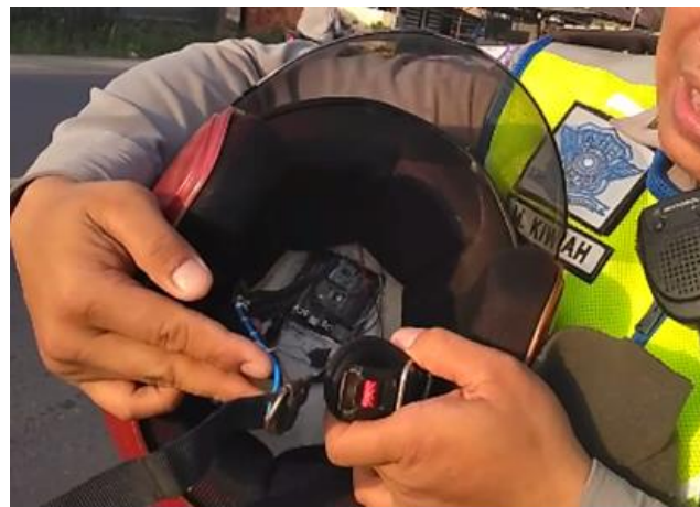
Figure 8. Electronic devices embedded at helmet unit.
