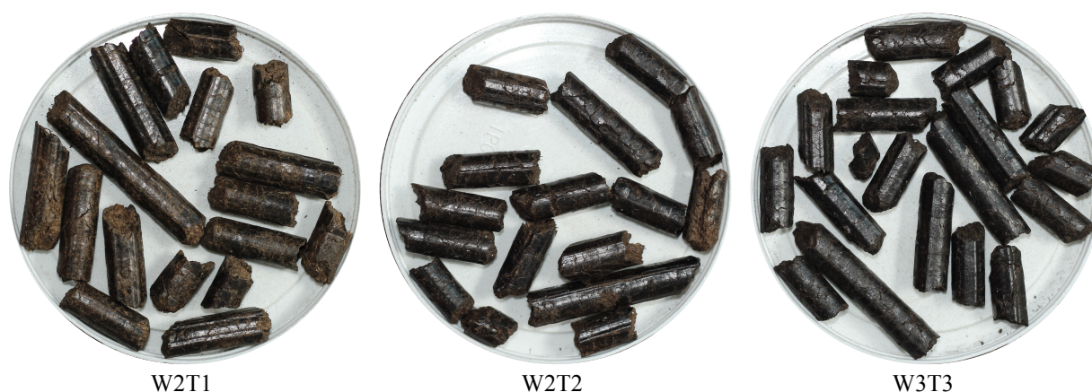
Figure 3. Example of torrefied pellets with torrefaction duration of 10 min (T1), 20 min (T2), and 10 min (T3)
