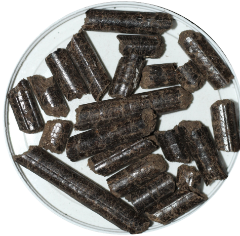
Figure 1. EFB Pellet used in the experiment
