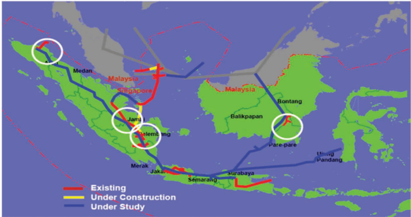
Gambar 1.2. Jaringan Pipa Gas Nasional
