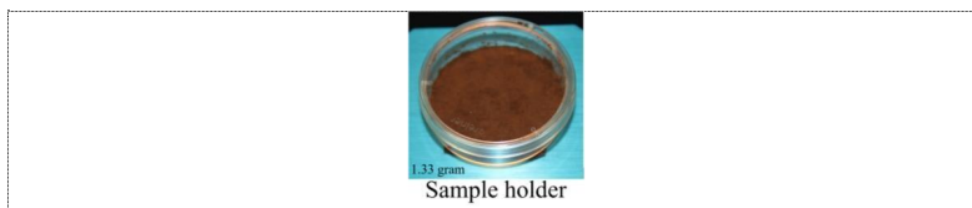
Figure 1. Sample holder for direct NIR spectral acquisition of ground roasted coffee using two handheld spectrometers equipped with an integrating sphere in the range of 650-1650 nm.
