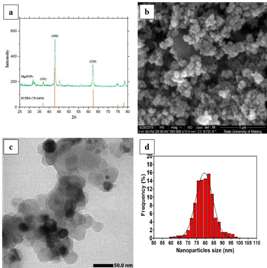
**Figure 3.** (a) diffraction pattern, (b) SEM image, (c) TEM image and (d) particles size distribution of synthesized MgONPs
