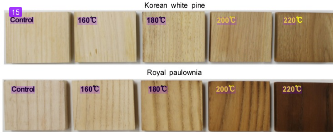
Fig. 2. Colors of Korean white pine and royal paulownia woods before and after heat treatment with the clamps at different temperatures.
