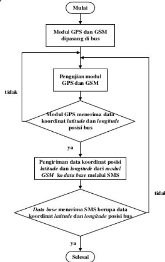
Gambar 2. Diagram Alir Sistem *Tracking* Bus
