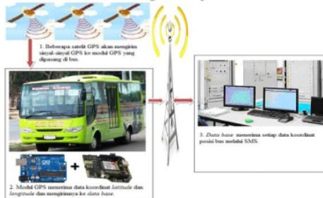
Gambar 1. Sistem *Tracking* Bus
