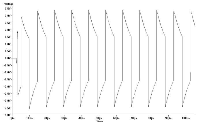
Fig. 8. Output Signal of Negative Clamp Biased Layout
