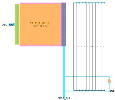
Fig. 5. Negative Clamp Biased Mask Layout
