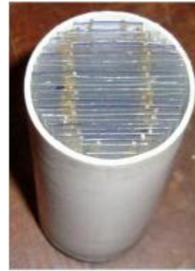
Figure 2. Parallel plate stack made of mica plastic sheets. The spacer between plates are nylon fishing lines. The stack casing is 1-1/4" PVC pipe.
