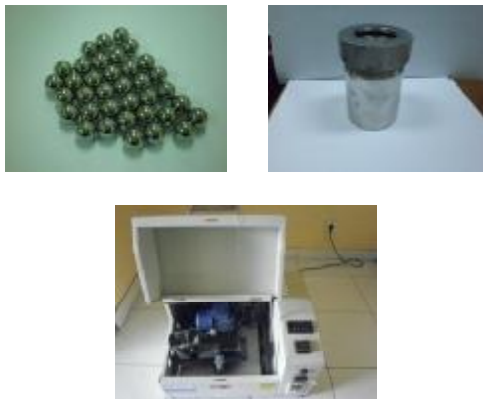
Fig. 3. Mechanical alloying tools (a) steel balls (b) vial (c) HEM-high energy ball milling
