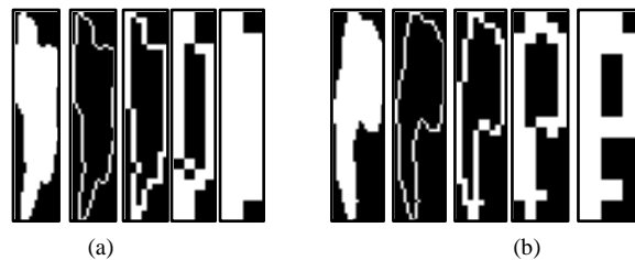
Figure 5. Example of covering results from the box-counting method. (a) Snowflake by camera A; raw image by 2DVD (leftmost), boundary covered by boxes of size 1, 2, 4, and 8; (b) Snowflake by camera B.
