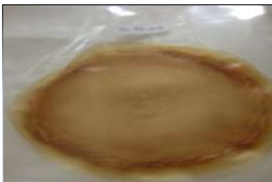
Fig. 1. Bioplastic with ratio starch-chitosan-filler formulation 7,5 : 2,5 : 0,25 (g/g).
