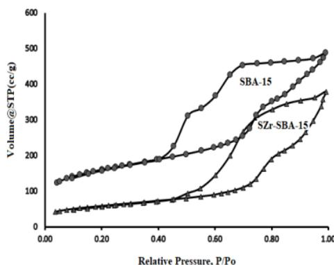
Figure 1. Adsorption-desorption curves of SBA-15 and SZr-SBA-15
