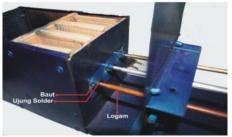
Figure 4. Metal connector and the box
