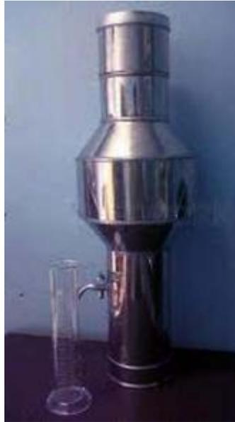
**Gambar 2.7** Alat ukur curah hujan (Ombrometer)
