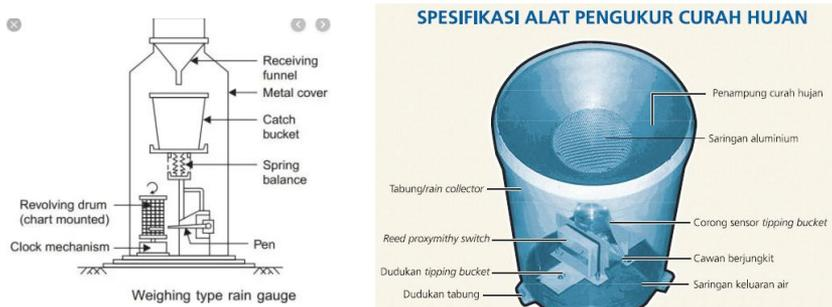
**Gambar 2.8** Alat pengukur curah hujan (Bucket Rain Gauge dan Tipping Bucket)
