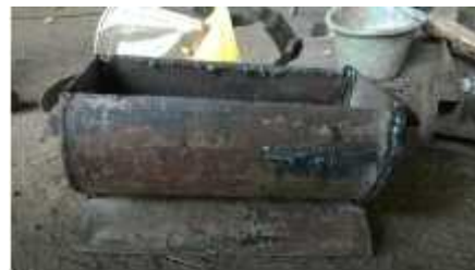
Figure 3.2 Crucible (galvanized container)
