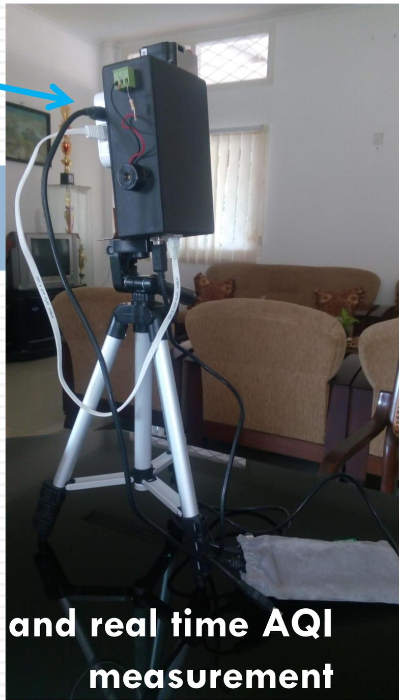
**On line and real time AQI measurement**
