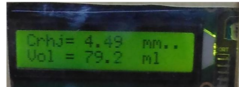
Fig. 6. Rainfall data shown on LCD layer
