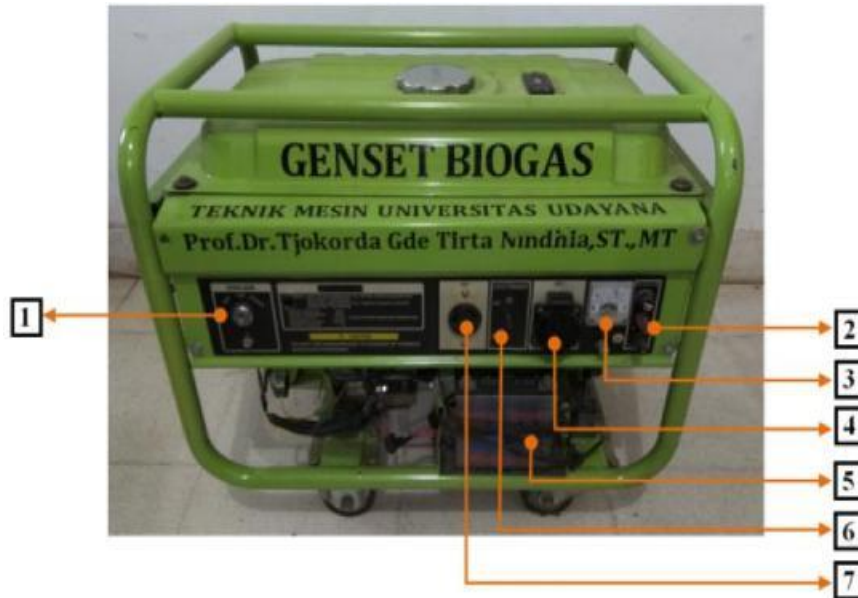
Figure 3. Biogas-fueled genset used in the experiment. Boxed numbers: 1. Ignition key, 2. DC 12 Volt output, 3. Volt meter, 4. AC output plug, 5. Battery 12 V, 6. Circuit breaker, 7. Three leg AC output plug.
