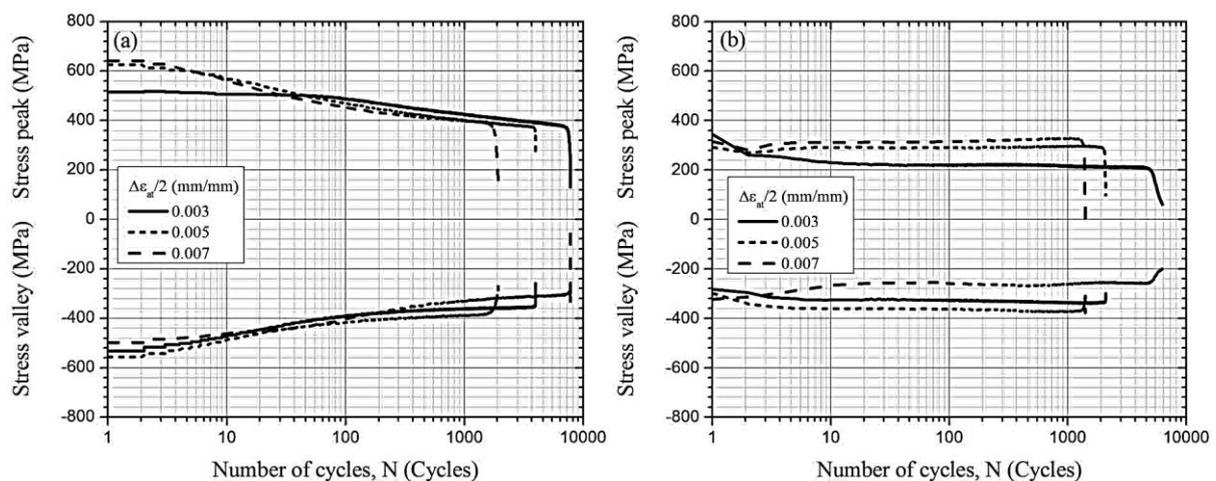
**Figure 3.** The cyclic stress responses of (a) CDS 1018 and (b) HDA steel with respect to the number of cycles at different strain amplitudes
