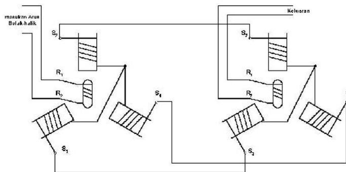
**Gambar VIII.31 Synchro error detector.**
