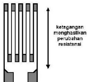
Gambar VIII.27 *Strain gauge*.
