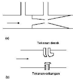
Gambar VIII.35 Meter aliran Dall: (a) tabung, (b) orifice.
