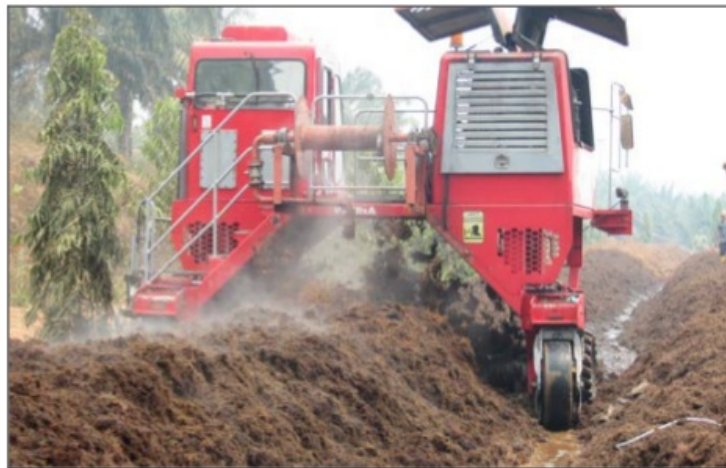
Fig. 3. High evaporation from a composting pile during turning operation
