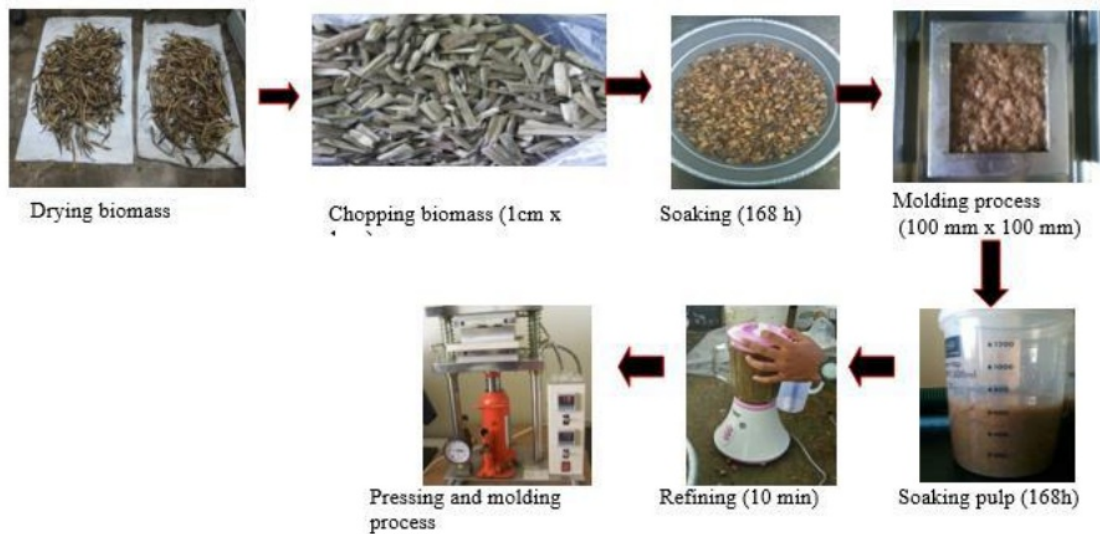
Fig 1: Biodegradable board producing process
